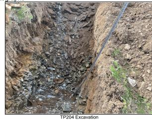
Remarks: Unable to advance the hole further than 1.50m. No groundwater encountered. On completion trial pit was backfilled with arisings.
