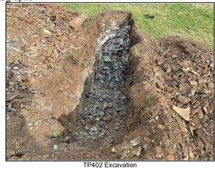
Remarks: Unable to advance the hole further than 1.10m. No groundwater encountered. On completion trial pit was
